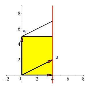
Finally, the area of the rectangle is (4)(5), which is also the determinant of F.
