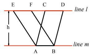
The area of a parallelogram is the product of its base and height. Since both parallelograms have base AB and height h, they have equal areas. So if we think of the side AB of the parallelogram as fixed and the opposite side as sliding along the line l, we see that all such parallelograms have equal area. We record this fact:
