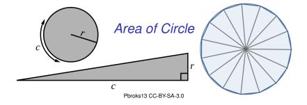
If C > T, where area circle = C and area triangle = T then inscribe a polygon inside the circle with area P so that T < P < C. Dissect the polygon into triangles. The height will be less than the radius and the sum of the widths (perimeter) will be less than the circumference because it is inside. Hence P < T, which is a contradiction to T < P.
