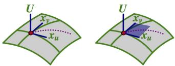
• Regular surface  $M = \mathbf{x}(u, v)$ , where  $\vec{x}_u \times \vec{x}_v \neq 0$ , and u(t) & v(t) give curve  $\alpha(t)$ . Then  $\vec{x}_u, \vec{x}_v$  form basis for  $T_pM$  and  $\alpha'(t) =$
