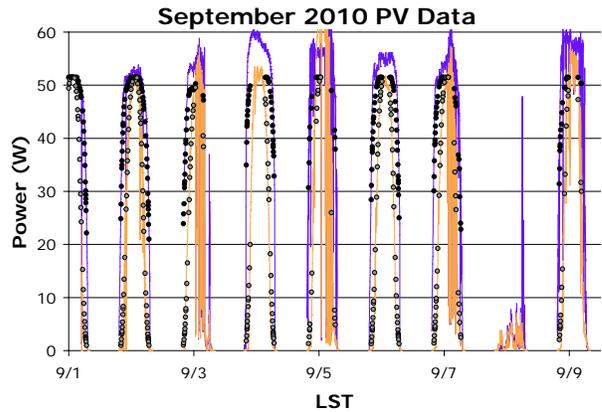
Fig. 11: Modeled performance plotted over measured performance time series.
