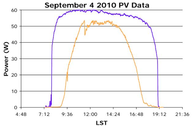
Fig. 6: Power produced by the tracking panel vs. the fixed panel. Integration reveals that tracking led to 79% more energy production over the day.
