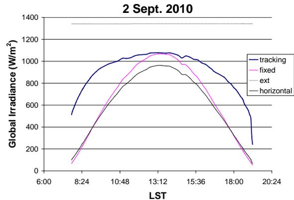
Fig. 9: Modeled irradiances incident on a tracking plane, fixed plane, horizontal plane and extraterrestrial based on AOD and water column using REST2.
