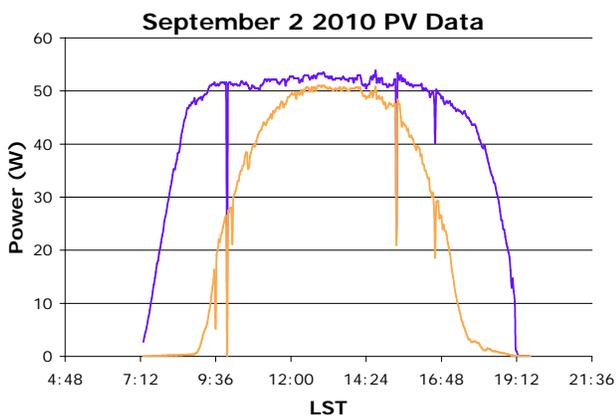
Fig. 5: Panel output power comparison for a relatively clear day. Tracking panel daily energy production was 64% higher than fixed panel. Sharp dips indicate quickly passing clouds.
