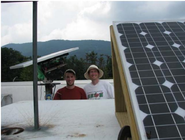
Fig. 4: Test site: fixed panel in foreground, tracker in background beside AppalAir atmospheric instruments [10].
