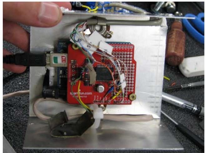
Fig. 2: Microcontroller interfaced with motor driver shield, motors, encoding pots and USB for program upload.
