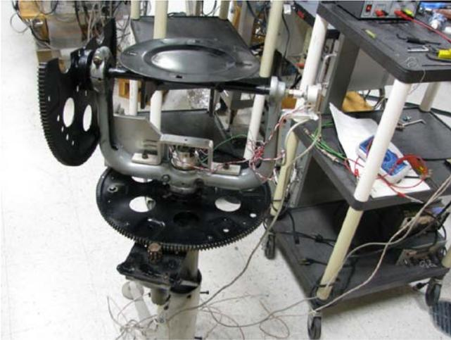
Fig. 1: Mechanical tracking system, showing automotive gears, pots, mount, and wiring for reading pot voltages.
