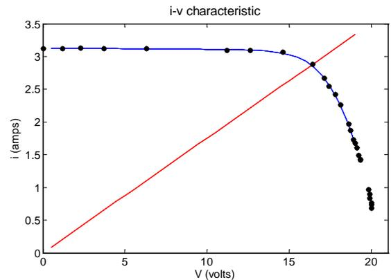
Fig. 3: Current-voltage characteristic of PV panels used, for global irradiance 944W/m<sup>2</sup>, temperature 30°C.
