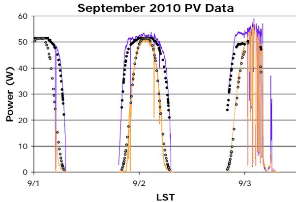
Fig. 12: Detail of model and measurement comparison, showing output behavior of PV panels driving fixed resistive loads.
