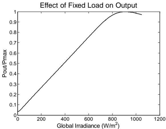
Fig. 10: Power out,  $P_{out}$ , varies in ratio with  $P_{max}$  with irradiance.  $P_{max}$  Watts would be obtained with a perfect MPPT tracking circuit.
